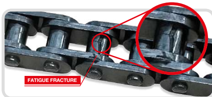
Photographed: A fatigue fracture induced by repeated loading of the chain against a worn camshaft sprocket, which in turn has caused localised structural damage to the chain bush.
